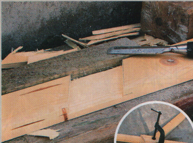
▲ Pic.1 Despite the scale drawings, Phil still likes to lay out the parts and check it's going to work. First stage is to mark out and cut the halving joints for the crosses. Glue and cramp these; leave to dry
