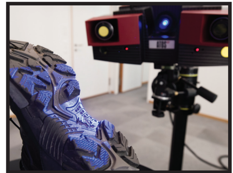
The ATOS 3D scanner and camera projects a moving fringe pattern on to the surface of an object using blue light. By combining information from the distortion of the fringe patterns, a detailed surface can be represented.
