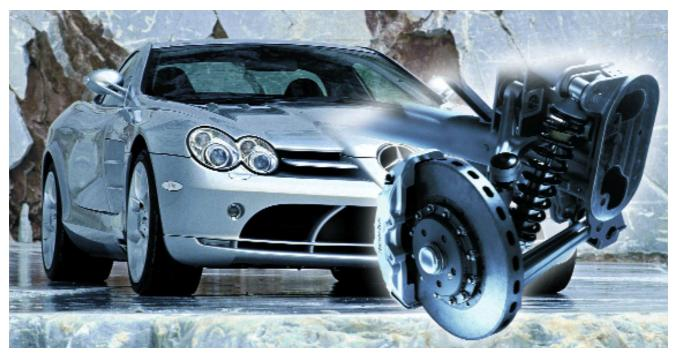
The Mercedes-Benz SLR uses fiber reinforced ceramic brake discs
