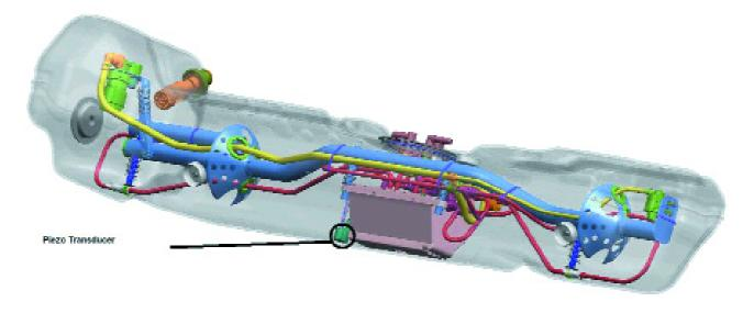
TI Automotive's new fuel level sensor uses a suspended piezoelectric ceramic material to send ultrasonic waves within the fuel tank
