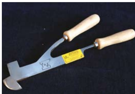
RAKING TOOL A raking tool is used to rake old caulking from between planks. This one can be struck with a hammer to help it along the seam
