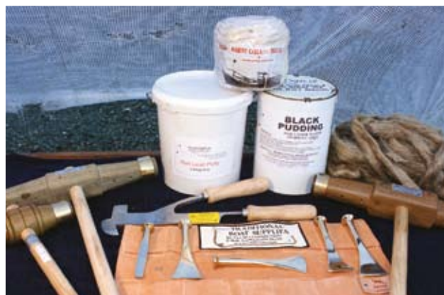
The caulker's toolbox consists of caulking irons, raking tool, mallets, cotton, hemp and stopping materials
