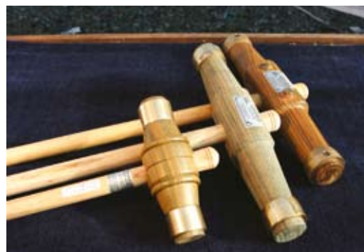
CAULKING Mallet The size of mallet depends on the the job being undertaken – the wider the seam the more force required so the bigger the mallet
