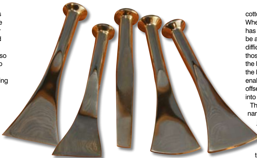
CAULKING IRONS The five irons to cover a spectrum of jobs are (from left) the standard making iron, the bent making iron, the king plank iron, the hardening iron for cotton and the hardening iron for oakum
