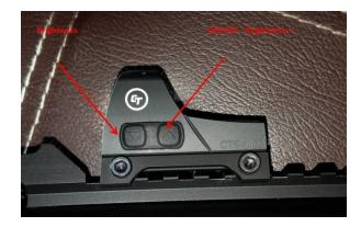
On the sight's left side you find the ON/OFF and brightness + and brightness – controls. They're
