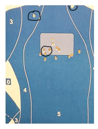
Out of the box the sight was shooting high, and I've circled those in black. I adjusted elevation and fired a 3 shot group, also circled in black, which was on the mark but needed a slight windage adjustment. I then fired two five shot groups which were right in there.
