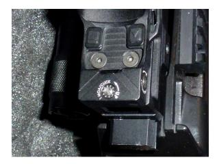
Looking at a top view, you'll see two arrow buttons. The up arrow activates the sight and progressively increases dot intensity with each press. The down arrow is used to turn off the sight or decrease the dot intensity. Accessing the brightness controls is easy and comfortable.
