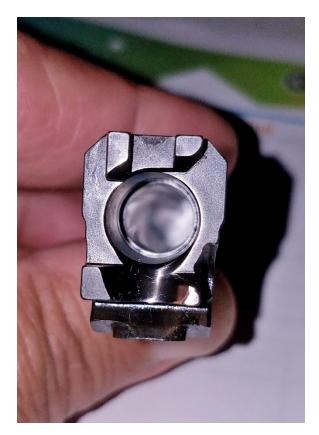
Equally impressive is the very clean polygonal rifling bore. After two hundred rounds at the range there were no visible signs of copper fouling.
