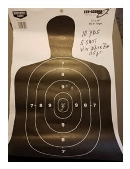
Winchester's USA Forged, steel cased 9mm 115gr ammunition resulted in a number of stuck cases and vertical stringing. It may be fine for your 9mm AR, but I can't recommend its use in a pistol; it's not even a good practice round.
