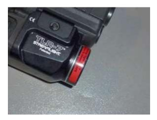
The head houses the LED electronics that drive the TRLR-7 to 500 lumens of well collimated white light. The light beam retains the characteristic well defined hotspot with an abundance of peripheral lighting that illuminates and average size room corner to corner.
