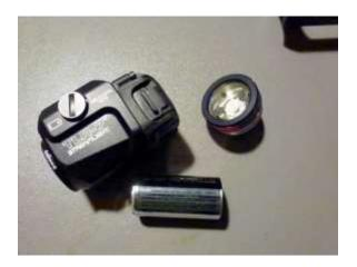
Installing fresh batteries requires removing the light's head from its housing to expose the battery compartment. The head which also functions as the battery cap is O-ring sealed to provide an IPX7 water resistance rating.
