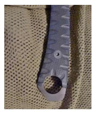
Moving down its full-length tang you see that it terminates in a wedge that can be used for prying.
